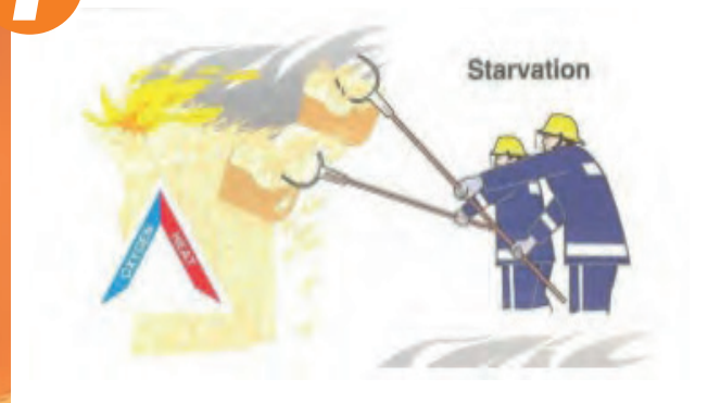
Removal of un-burnt material from fire area
